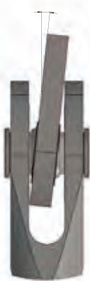
Additional misalignment with spherical bearing
